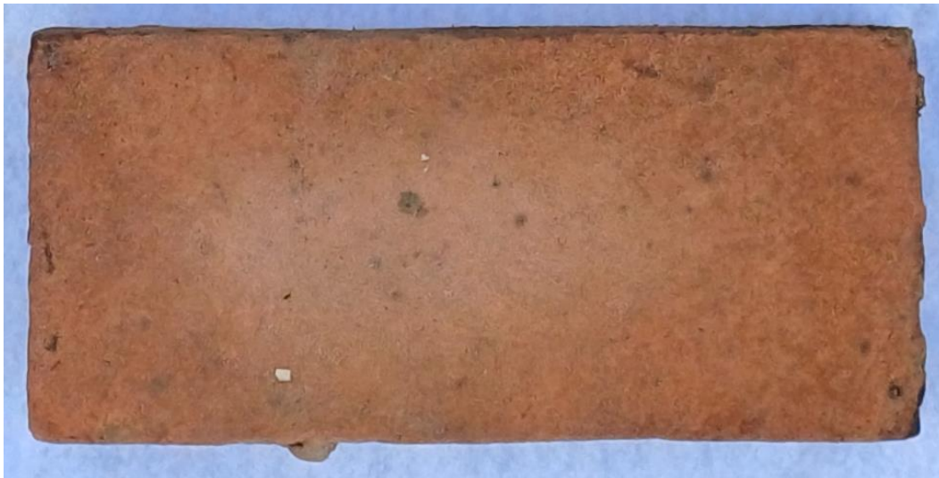
Image 7. The sharp edges and fine texture of this post-Civil War brick found at Pierre Almeras' brick yard on Old River indicates advanced technology equal to yards on Cedar Bayou. The bump on the bottom was caused when the still-soft brick was stacked at right angle on top of other bricks in the kiln. Image by author.
