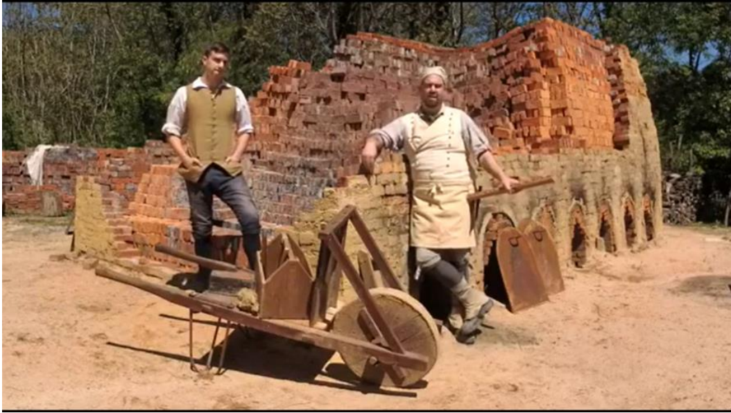
Image 10. This scove kiln at Colonial Williamsburg is identical to what was used at the Chambers County brickyards throughout the 19 th century. The tunnels to the right of the brick maker allowed wood to be charged into the kiln throughout the two-week burn. The dark bricks at the center burned hotter and harder and the brick shrinkage during the burn is evident in the picture. Screenshot from the Colonial Williamsburg production, Meet the Brickmakers!
