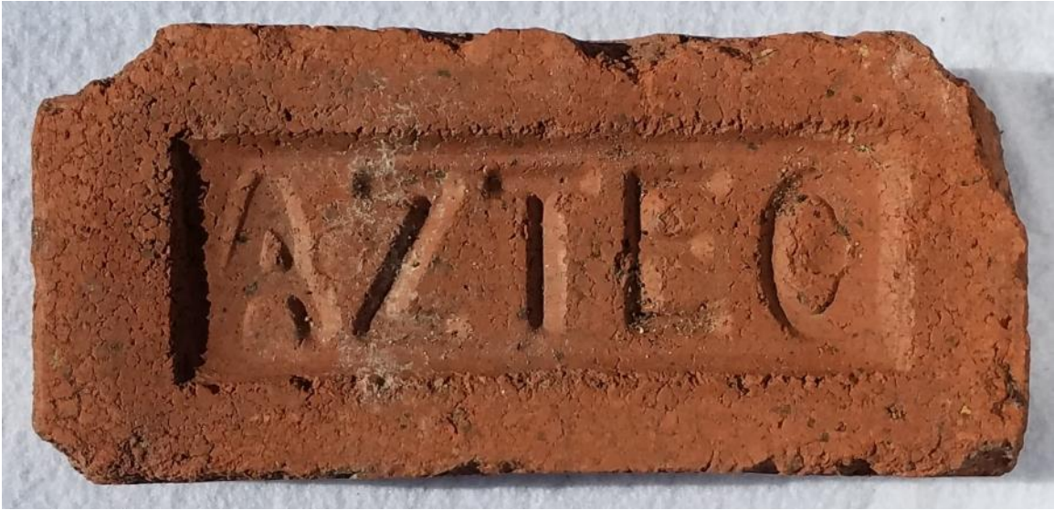
Image 18. This brick was found near the pond at the old Aztec brick plant behind Gene's Power Sports. The indentation carrying the brick logo is called a frog and was attached to the bottom of the brick mold by two screws. The impressions of the screw heads can be seen in this brick and also on the brick below. Image by author.
